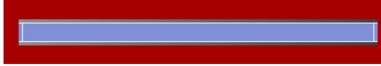
Figure 15 Connection of parts of type 1, (shown in blue) and 2 (shown in red). The loosening allows enough room for joining the parts by Tungsten Inert Gas (TIG) welding, but at the same time, it is possible to have good cohesion
