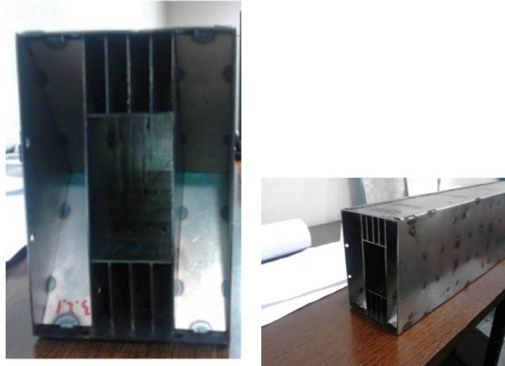
Figure 13 Section view of the welded beam (left) and its isometric view (right)
